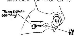
4a. Insert turnsignal assemblies into the fairing receptacles.
