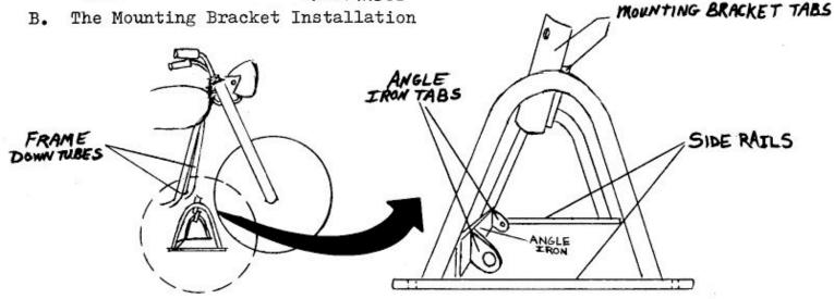
la. Start with the mount placed on the floor upside down (the side rails resting on the floor with the angle iron crossmember towards the rear of the bike).
