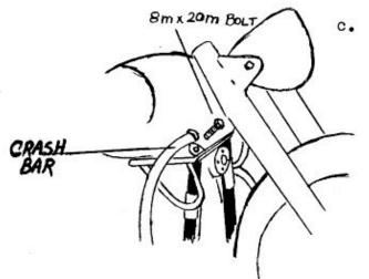
Use the 8mm x 20mm bolts provided to loosely bolt the two angle iron tabs onto the upper crash bar mount.
