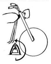
b. The mount is now carefully raised between the fender and the engine. Simultaneously, turn the bracket 180 degrees before it is raised to position beneath the crash bar.
