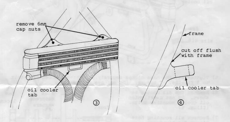
3) Lifting the oil cooler forward and up, remove it from the frame and let it hang to one side being careful not to damage any oil lines.
