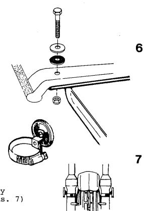
AFTER INSTALLATION, THE FAIRING OR BRACKET MUST NOT INTERFERE WITH ANY PART OF YOUR MOTORCYCLE, CHECK THE AREA BETWEEN YOUR MOTORCYCLE FORKS AND THE FAIRING FOR CONTACT AT ANY POINT (CABLES, HORNS, ETC.), WHILE TURNING THE HANDLEBARS COMPLETELY FROM SIDE TO SIDE.
