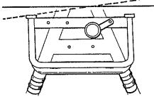
View the bracket from directly in front of the motorcycle. If the bracket is not level, tap it into position as required.
